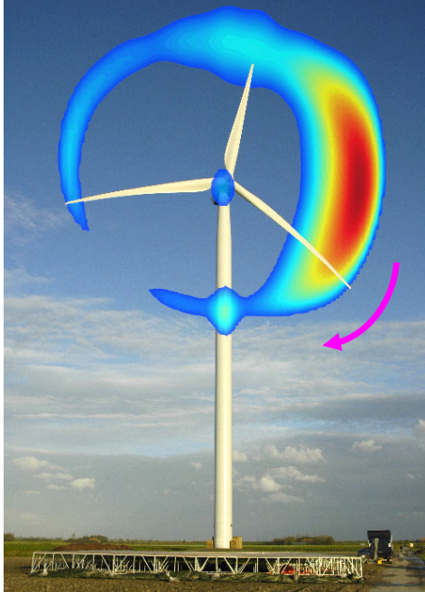
Figure 1: Noise source distribution in the rotor plane of a modern large wind turbine, measured about one rotor diameter upwind from the turbine. The source distribution is averaged over many revolutions. The range of the colour scale is 12 dB. Practically all noise is produced by the outer part of the blades (not the very tip) during the downward part of the revolution.
